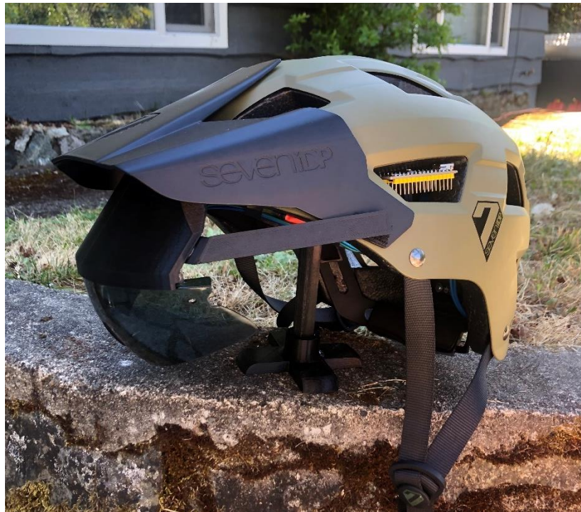
Figure 2: AR Bike Helmet Prototype Showing Visor, 3D Printed Parts, and Microcontroller.
